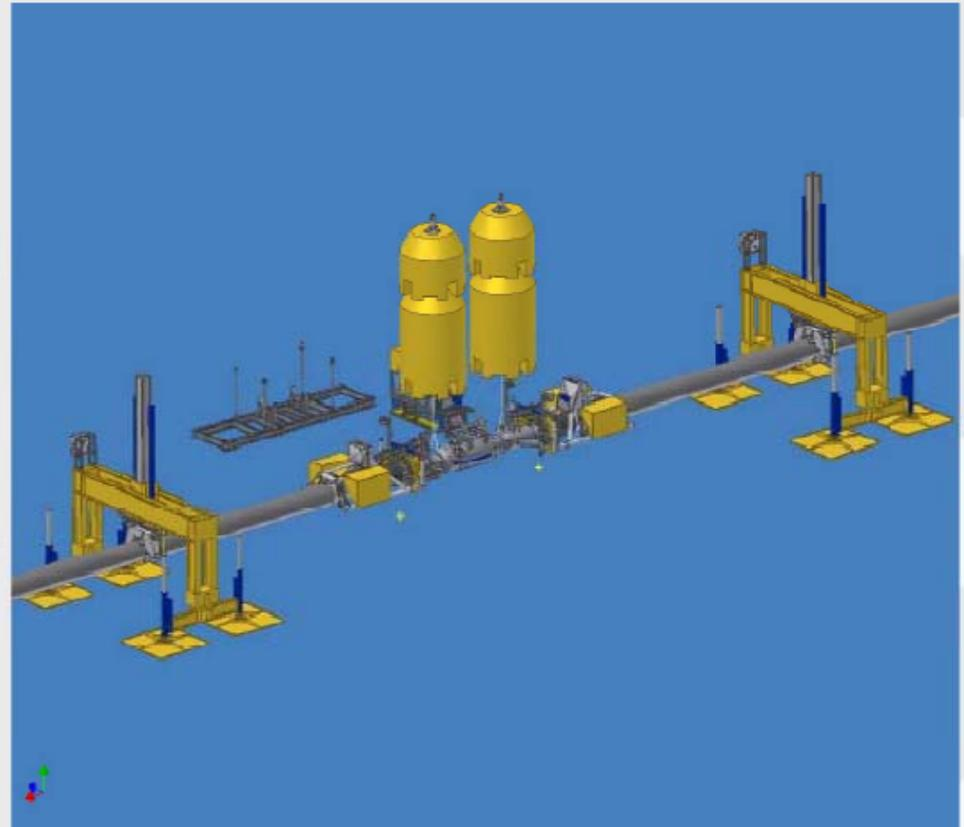
Saipem has stated that the system can be updated to 3500m by change-out of buoyancy and control pod
