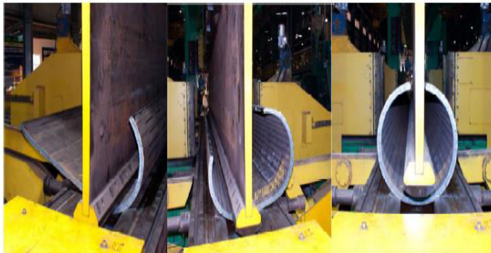
a) "J-ing" Stage b) "C-ing" Stage c) "O-ing" Stage JCOE Pipe Forming at JindalSAW, India (2012)
