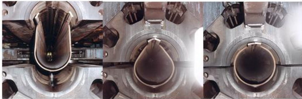
World Strongest : "O" Press Max Pressure force : 50,000t
