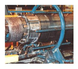
Corus Tubes UK UOE Mill has the strongest tooling in the world ensuring the required roundness and material compressive strength necessary for ultradeepwater line-pipes
