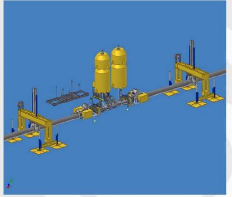
Saipem has stated that the system can be uprated to 3500m by change-out of buoyancy and control pod
